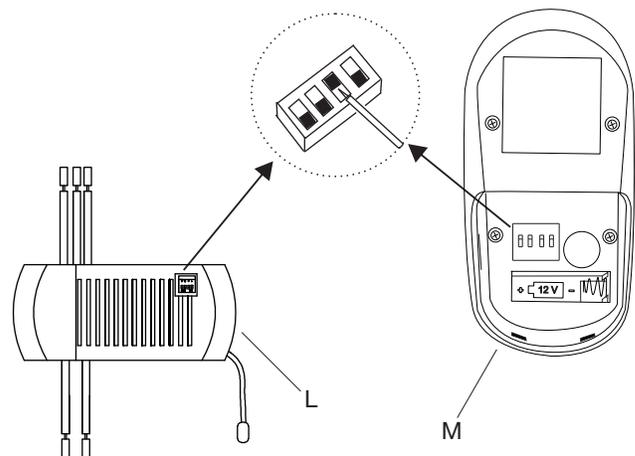
This remote control unit is equipped with 16 code combinations to prevent possible interference from or to other remote units. The frequency switches on your receiver (L) and remote control (M) have been preset at the factory. Please recheck to make sure the switches on the remote control (M) and the receiver (L) are set to the same position. Any combination of settings will operate the fan as long as the remote control (M) and receiver (L) are set to the same position.
