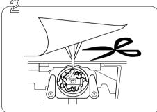
Cut the entangled thread with small scissors above the needle plate and then gently remove the thread and fabric.
