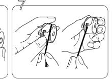
Pull the thread tail into the bobbin case groove, under the spring clip and into the thread guide hole.
