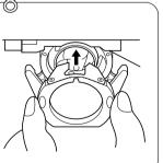
Insert the retaining ring with the notch up.
