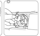
Holding the bobbin case by the latch align the finger with the top opening of the shuttle race, insert the case into the shuttle race and release the latch. The
