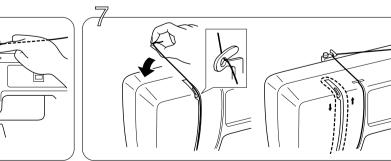
Guide the thread up the left channel, clear to the back of the opening around the take-up lever and back down the left side of the channel to thread the take-up lever.
