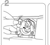
Raise the needle to its highest position, pull the latch and remove the bobbin case.
