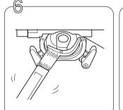
Remove any accumulated lint and thread with a brush.
