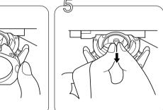
Remove the hook by grasping the center post and pulling out. Note it's position related to the driver.
