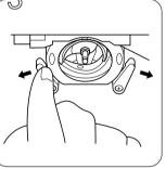
Slide the latch levers out from the retaining ring.
