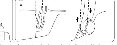
Pass the thread into the thread tension discs or \*behind the thread tension dial from the right to the left.
