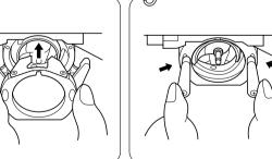
Push the latch levers into their locked position. Replace the bobbin cace. (See A.)
