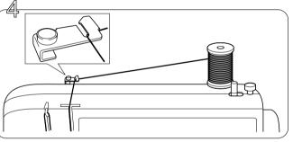
Pass the thread through the thread guide and down the right channel on the front of the machine.
