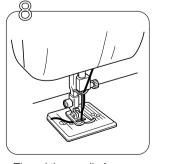
Raise the thread takeup lever to its highest position by turning the balance hand wheel.
