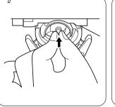
Grasp the center post of the hook, match the hook position opposite the driver and insert.
