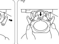
Remove the retaining ring.
