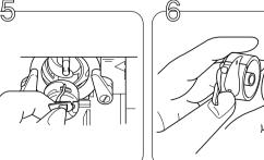
Raise the needle to its highest position and remove the bobbin case by pulling the latch.
