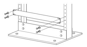
4 Use an equipment lift to align the chassis rack-mount holes with the equipment rack holes, and situate the chassis on top of the equipment rack bar.
