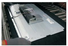
S14 Put the panel module on a protective cushion, then disconnect the panel lamp cable from the connector of panel module, then unplug the LVDS cable from the connector of the panel module.
