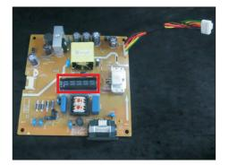
S20-1 Cut the glue between bulk cap. and PCB with a knife.
