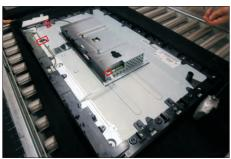
Take away the middle bezel, and put it on a fixture, then tear off the mylar tape for releasing the LED
