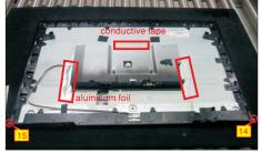
Use a Philips-head screwdriver to remove 13pcs
