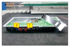
Use a Philips-head screwdriver to remove 5pcs screws for unlocking the power board and interface board, and then release all the cables from the hooks.
