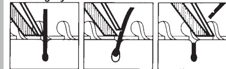
Groove channels beard closer to cutting system Lifter raises hair Blade cuts hair which then drops below skin level
