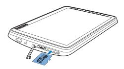
1 Open the cover of the Micro SD card slot.2 Insert the SD card into the slot until it is
