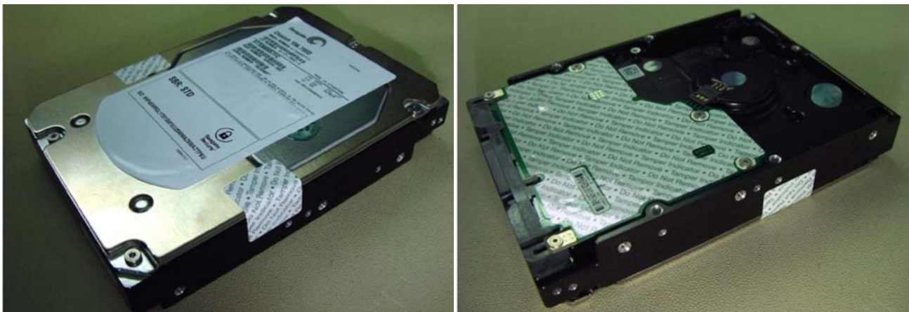
Figure 10. Example of FIPS tamper evidence labels.
