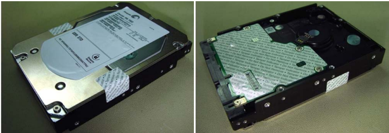
Figure 7. Example of FIPS tamper evidence labels.
