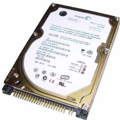
Figure 1. Momentus 5400.2 Blade Server PATA disc drive
