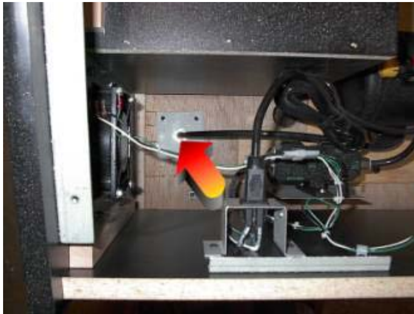
Figure 1 Top View - Drain from tank
