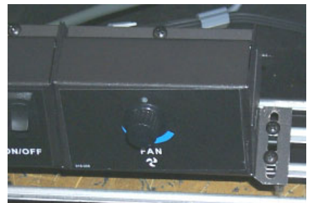
Secure right side with 2 screws.
