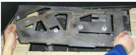
Slide the burner to the left and lift out.
