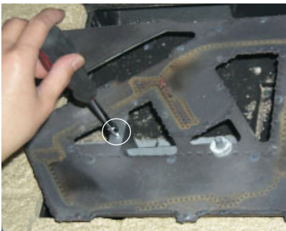
Remove the screw on the left side of the burner.
