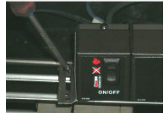
Secure left side with 2 screws.
