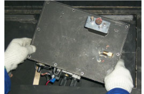
Lift entire valve tray assembly out.
