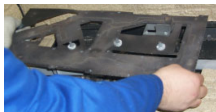
Diagram 1: Remove the left screw and then slide the burner assembly away from the orifice and lift out.
