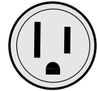
Two-Pole, 3-wire Grounding Receptacle 15 Amps. 125V.
