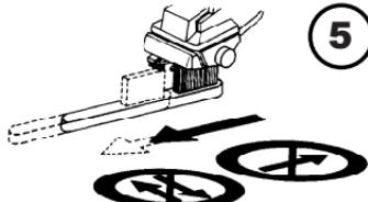
Use the supplied brush to clean the stylus and dynamic stabilizer. Brush only from back to front, as shown ⑤. Do not use liquids on the stabilizer brush. Use alcohol or an alcohol-distilled water solution to clean the stylus. Commercial cleaning solutions may damage the stylus.
