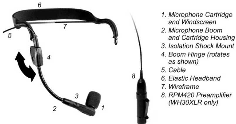
WH30 HEADSET MICROPHONE PARTS FIGURE 1
