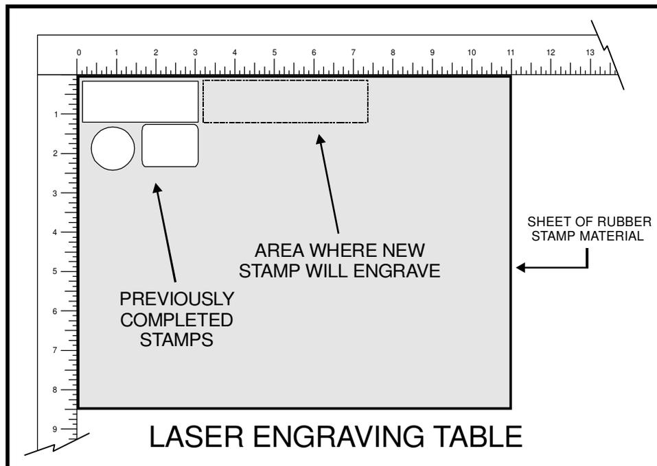
Place a sheet of rubber stamp material into the **UPPER LEFT CORNER** against the rulers, as the following diagram illustrates, and be sure to properly focus on the material. Now, set the printer driver settings as shown on the following page.
