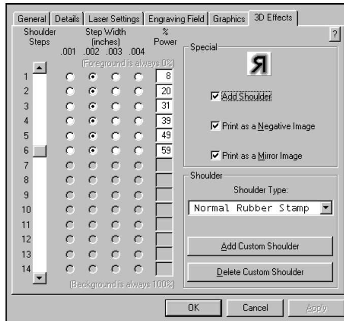
Print to the laser system. Position the full sheet of rubber stamp material in the same upper left location on the engraving table and begin engraving. The driver automatically adds the shoulder, mirrors the entire page, and creates a negative image for engraving, and cuts out the stamps.
