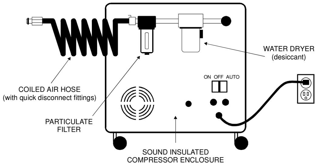
Please refer to the instructions supplied with the Air Assist Compressor on how to properly install and use this option.
