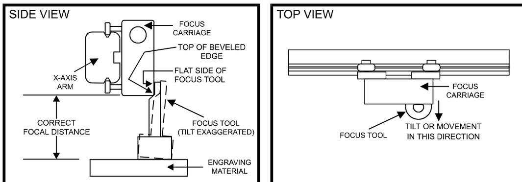
Remember, having the cursor, in the display, located on the tenths digit will move the table quickly and having it on the hundredths digit will move it more slowly. After focus has been established, remove the focus tool and press the "Z" button to move the focus carriage back into the home position.
