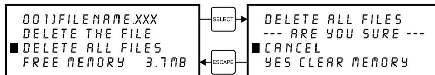
To completely clear out the entire memory buffer all at once, use the up and down arrow keys to position the cursor on the "DELETE ALL FILES" option and press the "SELECT" button. The laser system will again ask if you are sure so respond accordingly.
