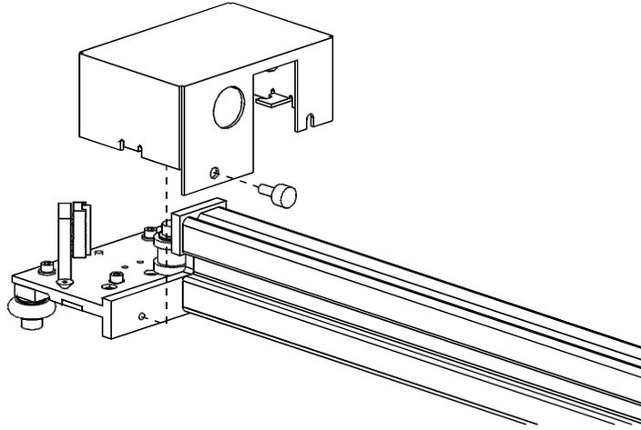
Inspect the #2 Mirror and clean it only if there is debris present. There are two ways to clean the mirror, with a moistened cotton swab or a moistened lens tissue.
