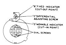
These controls have an adjustable differential. The movable indicator points to the temperature at which the compressor starts. The fixed indicator points to the temperature at which the compressor will stop. The difference between these two indicators is the differential.
