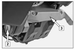
Remove the lower screw [2] on the right tank. Remove the HH screws and take off the battery cover [3].
