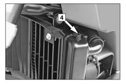
Remove the bleeder screw [4] on the left side of the radiator.
