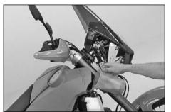
To be able to completely bleed the cooling system, raise the motorcycle approx. 50 cm in the front.
