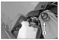
Carefully remove the radiator cap [2] with a rag, turning in a counterclockwise direction. The radiator should be completely filled with cooling liquid. No air should be in the radiator.
