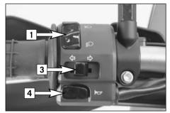
ФФ The indicator switch [3] returns to central position after actuation. Press flasher switch towards switch housing to switch off the flasher.
