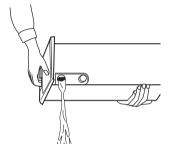
The water reservoir has a capacity of approx. 3.8 litres. This is sufficient for a laundry load of 5 kg which has been machine spun at 800 revolutions per minute.
