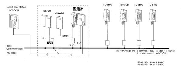
TD-H/A multiple-station is capable of connecting PanTilt door station, in conjunction with DE-UR adaptor. For long-distance application, locate MYW-BA adaptor between PanTilt door station and MY-CU monitor.
