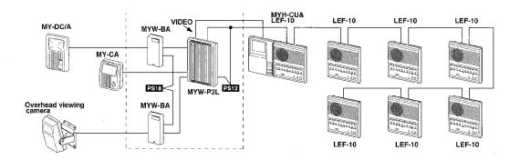
The above example illustrates 2 PanTilt door stations and an overhead viewing camera MY-CA (in MYW-CA) are connected to 7-call LEF-10 system.
