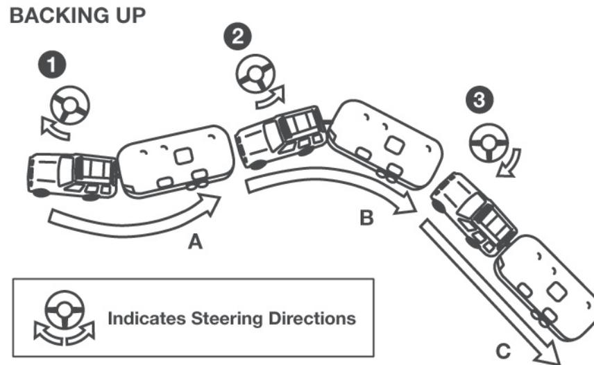
Position (A) start. Turn steering wheel as shown in (1) will put you in trailer Position (B). Turning steering wheel show in position (2) puts you in trailer position (C). Steering position (3) returns front wheels for straight backing.
