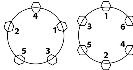
NOTE: Use a torque wrench to tighten lug nuts. Tightening by hand or with an impact wrench is not recommended.
