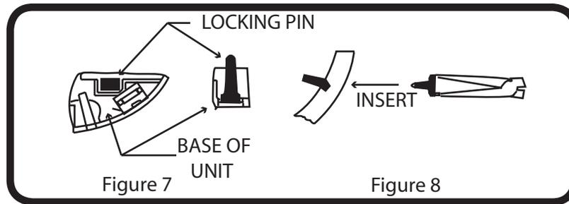
1. Remove the breakaway locking pin from the unit by rocking pin back and forth.
