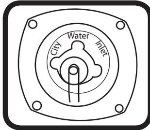
After hooking up the hose and turning on the city water valve provided in the park, slowly open a faucet. There will be a lot of spurts and sputtering until all the air is expelled from the trailer system. If the water heater and fresh water lines are empty it will take some time before all the air is expelled and you get a steady flow of water at the faucet. Once a steady flow is achieved at one faucet the others should be opened long enough to expel the air in the lines going to them.
