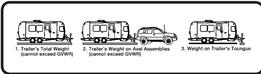
When loading heavy objects such as tools, skillets, irons, and boxes of canned goods, etc. keep them as low as possible - preferably on the floor. Try to hold additional weight behind the axle to a minimum.
