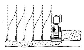
Leave material which drifts over side of bucket for final clean-up.
