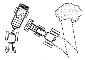
To increase loading efficiency, minimize angle of turn and length to run between pile and spreader.
