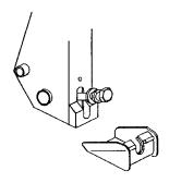
9. Raise the loader and lock the support stand tubes into the up position.
