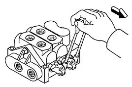
Work both levers back to direct pressure to both cylinders.
