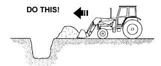
When backfilling, approach pile with a flat bucket. Leave dirt in bucket. Dumping on each pass wastes time.
