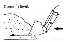
NOTE: Bottom surface of bucket is parallel to line on motion.
