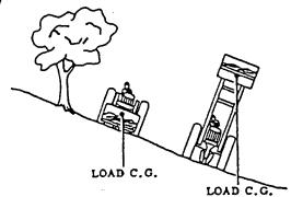
Do not raise bucket to extreme heights while tractor is on an incline. Carry loader low for safety. Note in above illustration how the center of gravity moves out when bucket is raised on a slope. Be alert for terrain changes and adjust bucket accordingly. Keep bucket low, no more than one foot high, as long as possible.
