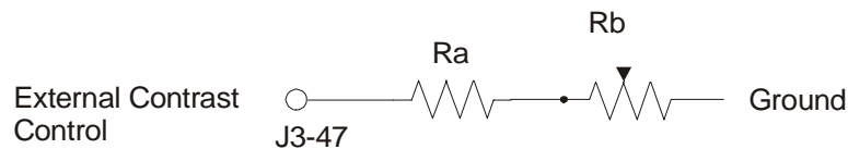
Figure 2–10. External Contrast Adjustment for LCD Panels
