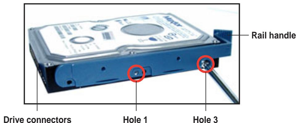
3. Attach **Rail 2** to the other side of the drive as shown. The rail end should be on the side of the drive connectors.
