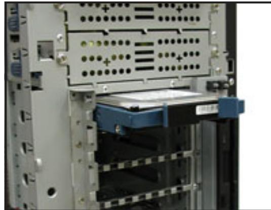
6. Push the drive all the way to the depth of the bay until the rail locks clicks, indicating that the drive is securely in place.
