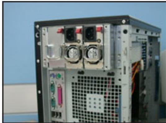
7. Secure the power supply to the chassis with two screws on each metal bracket.
