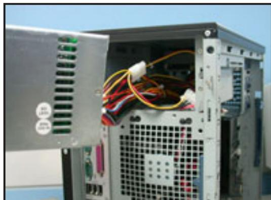
5. Push the power supply halfway to the power supply cage, then attached the a metal bracket on each side of the power supply with two screws.
