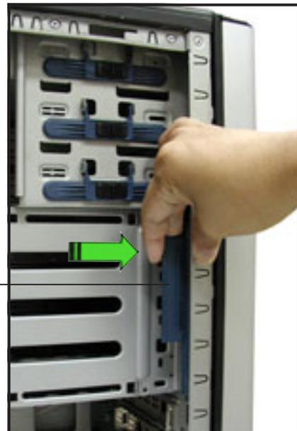
2. Pull and swing the left edge of the front panel outward.
