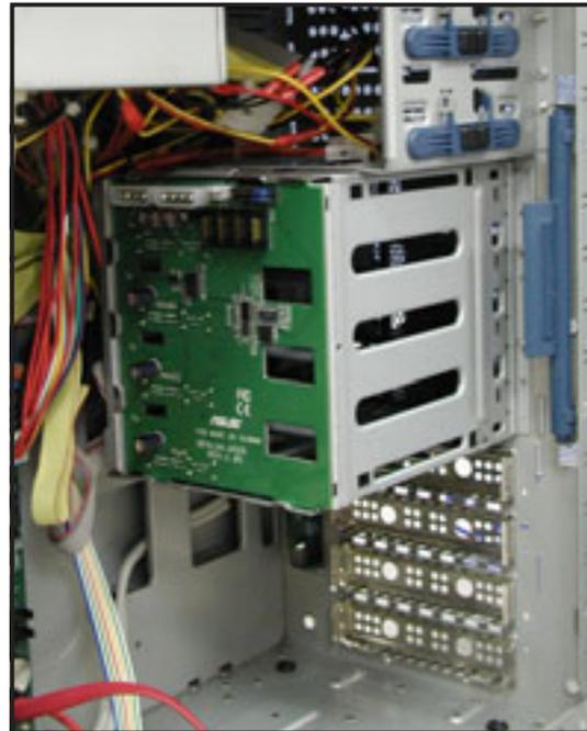
3. From the inner edge, push the backplane outward so that the outer edge protrudes slightly from the slot.
