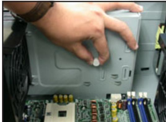
3. Locate and remove the metal stopper from inside the power supply cage.
