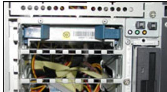
7. Connect the IDE and power cables to their corresponding connectors on the back of the drive.
