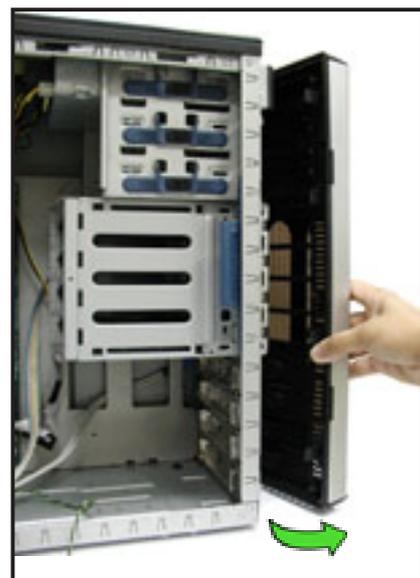
3. Unhook the hinge-like tabs from the holes on the right side of the front panel to completely detach the front panel assembly from the chassis.
