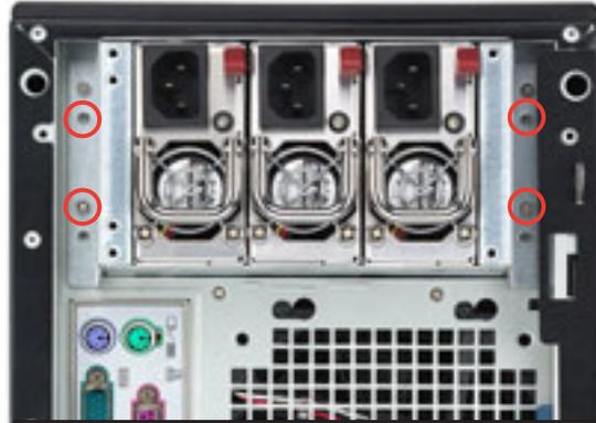
2. Use one hand to push the power supply module from inside the power supply cage, then carefully pull out the power supply module from the chassis.
