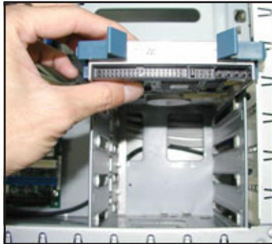
4. Connect the signal and power cables to their corresponding connectors on the back of the drive. Refer to the preceding sections for details.
