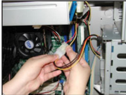
4. Connect one end of the supplied 7-pin SATA cable to the SATA connector at the back of the drive, then connect the other end to a SATA connector on the motherboard. Refer to the motherboard user guide for the location of the SATA connectors.
