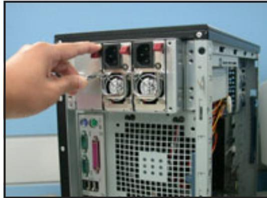
3. Secure the power supply to the chassis with two screws on the metal brackets on each side.
