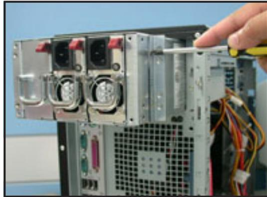
6. Push the power supply to the power supply cage until the metal brackets and the chassis screw holes align.
