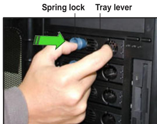
3. Firmly hold the tray lever and pull the drive tray out of the bay.
