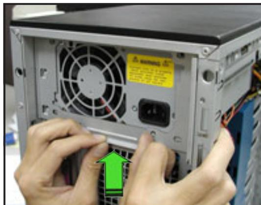
To remove a 600 W dual or redundant power supply:
