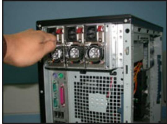
The pictures shows the power supply module when installed.
