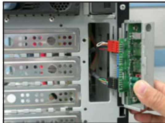
4. Remove the screw that secures the I/O board to the bracket.
