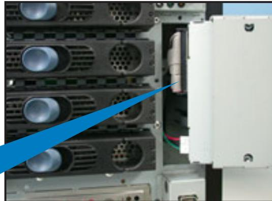
3. Carefully push the drive into the bay until the drive cage fits the front edge of the bay.
