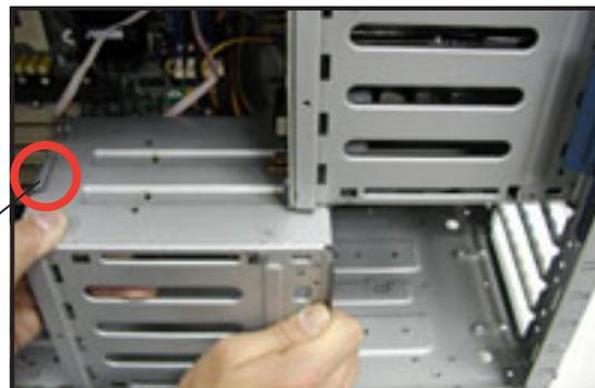
2. Carefully slide the drive cage toward the front panel until it fits in place.
