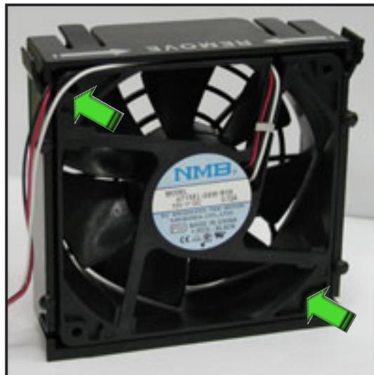
2. Firmly hold the chassis fan on the side with the tabs and position it into its slot, making sure that the four hooks underneath the fan match the corresponding holes on the rear panel.
