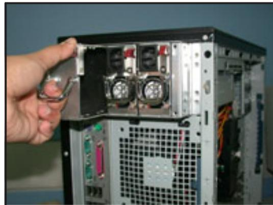
3. Insert the power supply module to the empty bay with the power connector on top.
