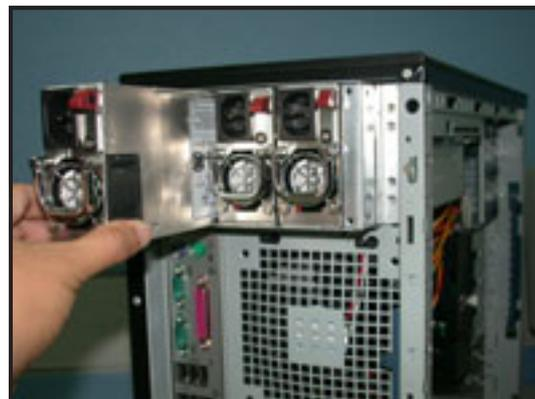
4. Push the power supply module inside the bay until it is aligned with the other power supply modules.
