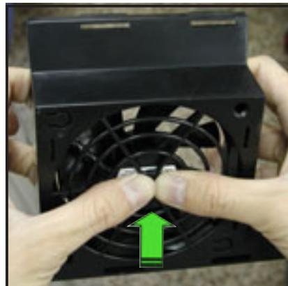
To re-install the HDD fan:
