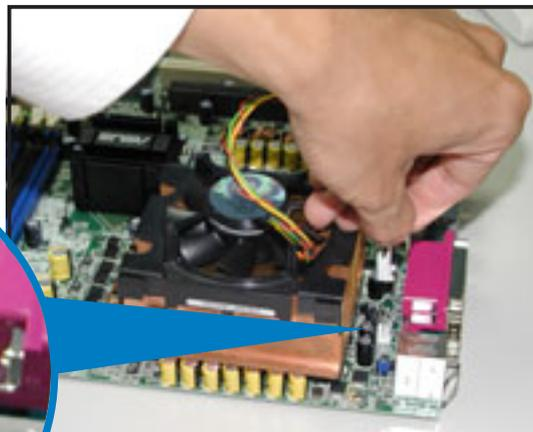
CPU1 fan connector (CPU\_FAN1)
