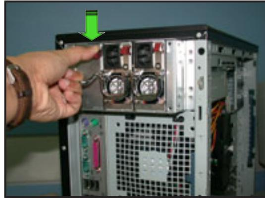
2. Use the module handle to pull the dummy module out from the power supply case.
