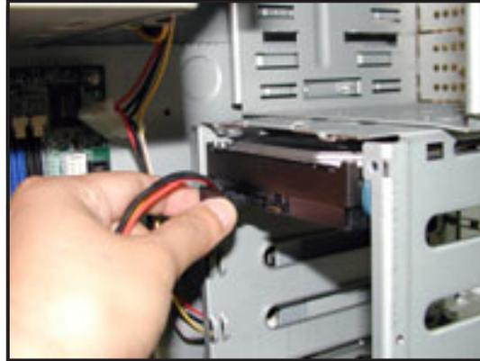
3. Connect the other end of the SATA power cable to a 4-pin plug (female) from the power supply unit.
