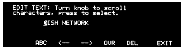
The text edit tools are indicated along the bottom of the screen: Case, Skip Back, Skip Forward, Overstrike/Insert, and Delete.
