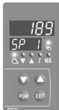
Figure 13D - Operation Set Point
