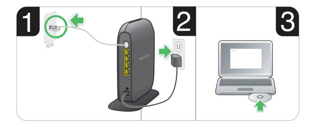
Connect your Router's ADSL cable to your ADSL connection. If you are replacing an existing Router or gateway, this may require unplugging the existing gateway.
