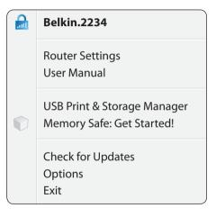
The Belkin Router Manager appears in your system tray (Windows) or menu bar (Mac). Its icon indicates the current status of your Router and also allows you to access your Router's settings to make changes. It also provides quick access to software that came bundled with your Router.
