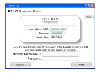
5. After a brief installation, the setup software will ask you for the network name and password from the network information card that is attached to your Router. Store the card under the base of your Router for future reference.
