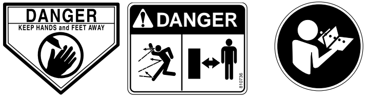
Label Danger Keep Hands and Feet Away Item 3 Part No.400424 Label Danger Flying Material Item No. 19 Part No. 810736 Label Read Owner's Manual Item 15 Part No.830301
