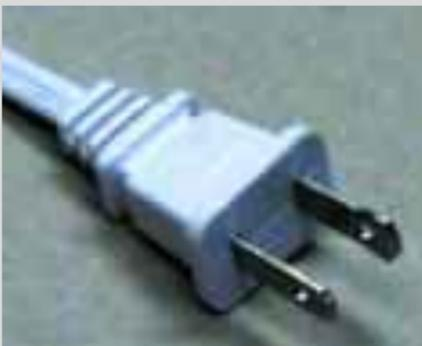
**THIS PRODUCT IS EQUIPPED WITH A POLARIZED AC (Alternating Current) PLUG (a plug having one blade wider than the other). This plug will fit into the power outlet only one way. If the plug does not fit fully into the outlet, reverse the plug. If it still does not fit, contact qualified personnel to install the proper outlet. DO NOT DEFEAT THE SAFETY PURPOSE OF THIS POLARIZED PLUG IN ANY WAY.**
