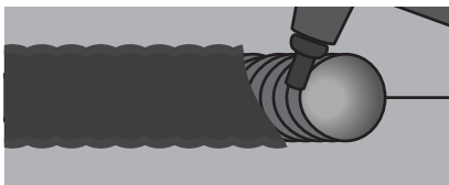
PARTIALLY CHIPPED AWAY TO SHOW WELD
