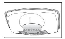
Operating temperatures are controlled by the setting knob (see diagram) located on the ceiling of fridge compartment. Settings may be made from min, 1 ... 6, max, max being the coldest position.
