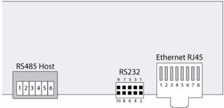
Fig. 7.1 Connectors on upper PCB
