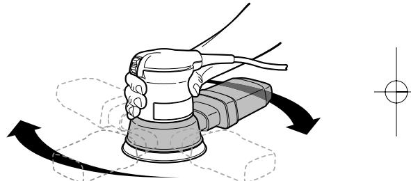
You may grip the tool on top or around the motor housing as shown, which was contoured for that purpose.
