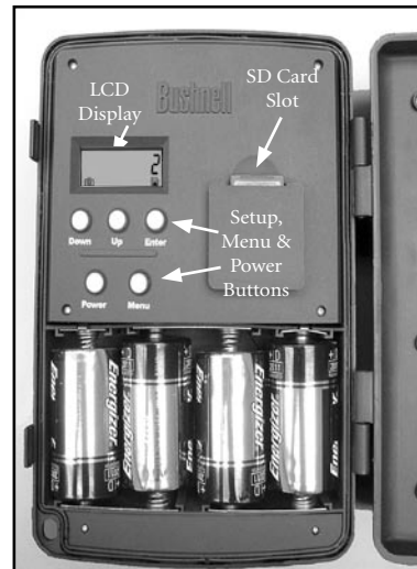
Control Panel Inside Front
