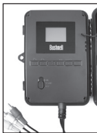
Cable from "A/V Out"
