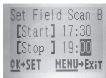
[Step 5] (opt)-set Field Scan “B” Stop & Start
