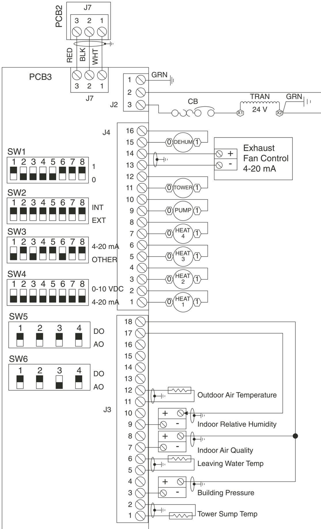
**50BV,XJ Accessory Control Module (PCB3) Schematic**
