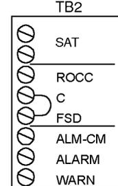
Fig. 2B — Field Terminal Block for 50BV Unit
