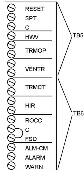
Fig. 2A — Field Terminal Blocks for 50XJ Unit
