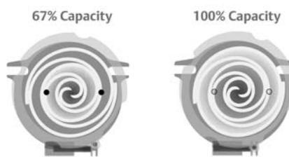
sealing the bypass ports and instantly shifting capacity to 100%. Take advantage of "shift on the fly" stage changing (no stopping and starting required like other two-stage compressors).
