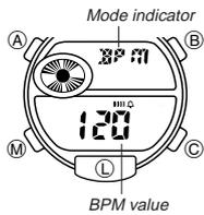
The Beat Counter Mode can be used to produce an audible signal in accordance with BPM (beats per minute) value, which is like a digital metronome that can be used for a variety of different musical applications.
