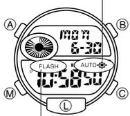
A backlight that uses an EL (electro-luminescent) panel causes the entire display to glow for easy reading in the dark. An auto light switch causes the EL backlight to turn on when the watch is angled toward your face for reading. An EL alarm feature can be turned on so the backlight flashes whenever an alarm or hourly time signal sounds.
