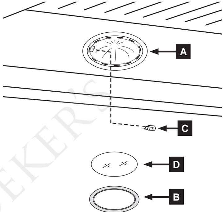
5. Center the lens **D** on the lens retaining ring **B** and snap it back into place on the light fixture **A**.
