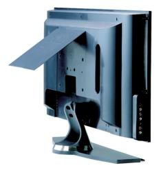
**3** Connect the white DVI cables and the audio cables.
