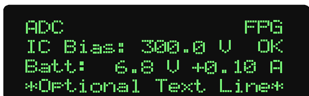
Figure 2-10. Test/Detector Screen 3 - Bias and Battery Voltages Plus an Option Text Line
