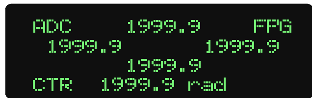
Figure 2-17. An Absolute Dose Measurement With Air Density Corrections and the Front Panel Gain Factors Enabled
