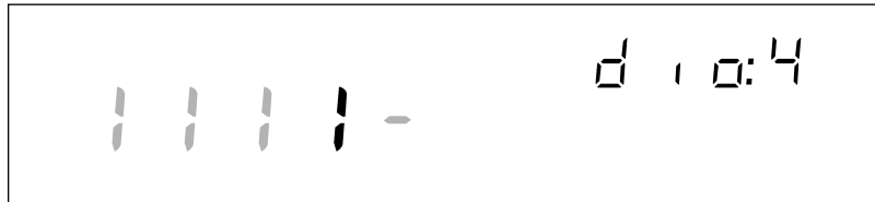
Digital I/O status display for DIO line 4 (for the example 1111 -0000 )
