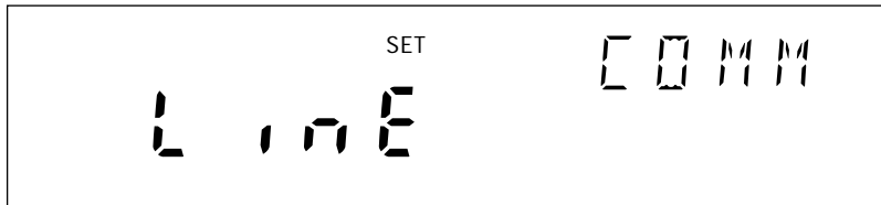
Communications display for setting the line frequency
