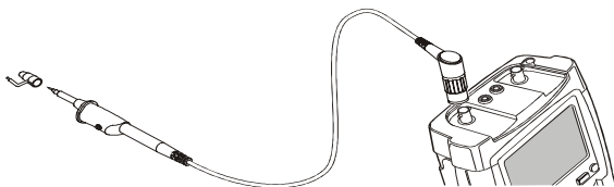
Figure 37. HF Voltage Probe Connection Using Ground Spring
