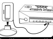
Snap AM antenna into provided stand, then plug antenna cable into socket on back of iP86. Move antenna 12" away. Extend FM antenna.
