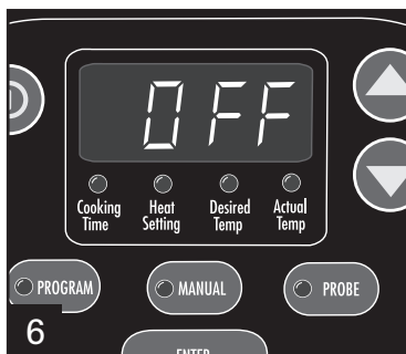
6 The unit will turn off and display OFF after a total of 14 hours.
