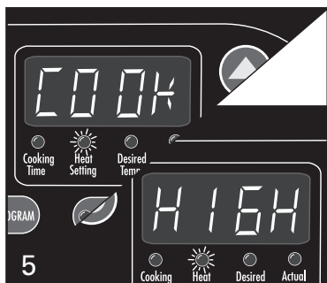
5 The display will alternate between COOK and heat setting (if HIGH or LOW is selected). If using Warm setting, display will remain on WARM.
