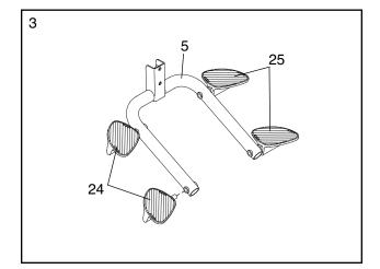
Orient the Pedal Frame (5) as shown, and then insert the Pedal Frame into the Pivot Frame (6).
