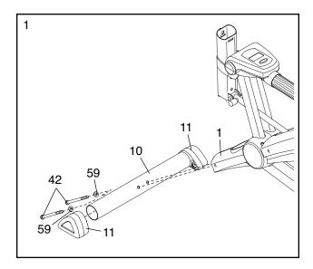
Press a Stabilizer Endcap (11) onto each end of the other Stabilizer (10). Attach the Stabilizer to the back of the Frame (1) with two M10 x 75mm Button Screws (42) and two M10 Curved Washers (59).
