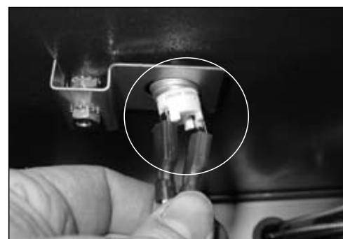
Figure 8.18 Connect the electrical connector to the snap disc.
