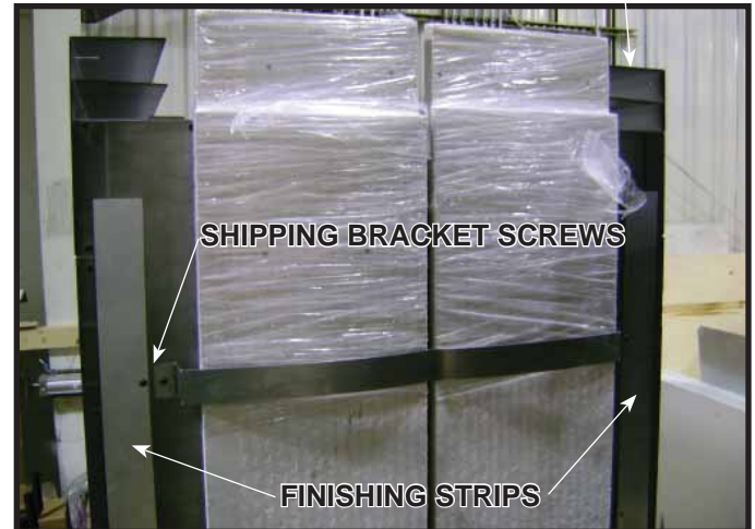
Figure 9.3 Shipping Brackets and Finishing Strip Locations.
