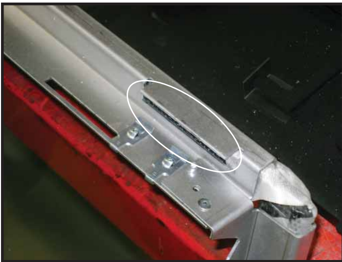
Figure 14.1 Glass Top Tab Detail.
