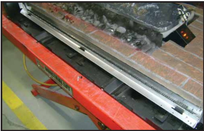
Figure 14.5 Bottom Glass Latch Tabs Installed in Glass Frame
