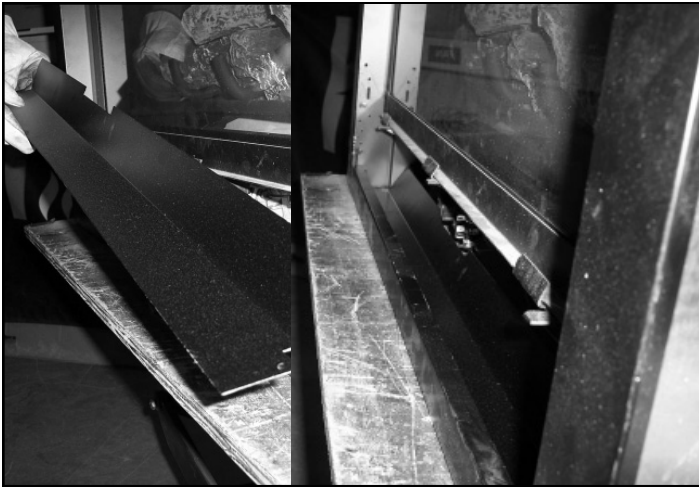
Figure 12.7 Installing Floor Cover
