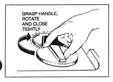
Always close the main cup tightly, but do not overtighten. When firmly latched, you will hear a clicking sound.
